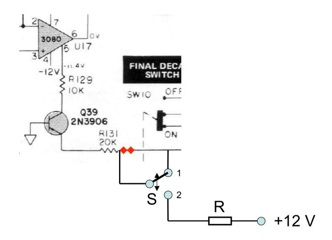
S: single-pole switch without middle rest i.e. "ON-ON"
